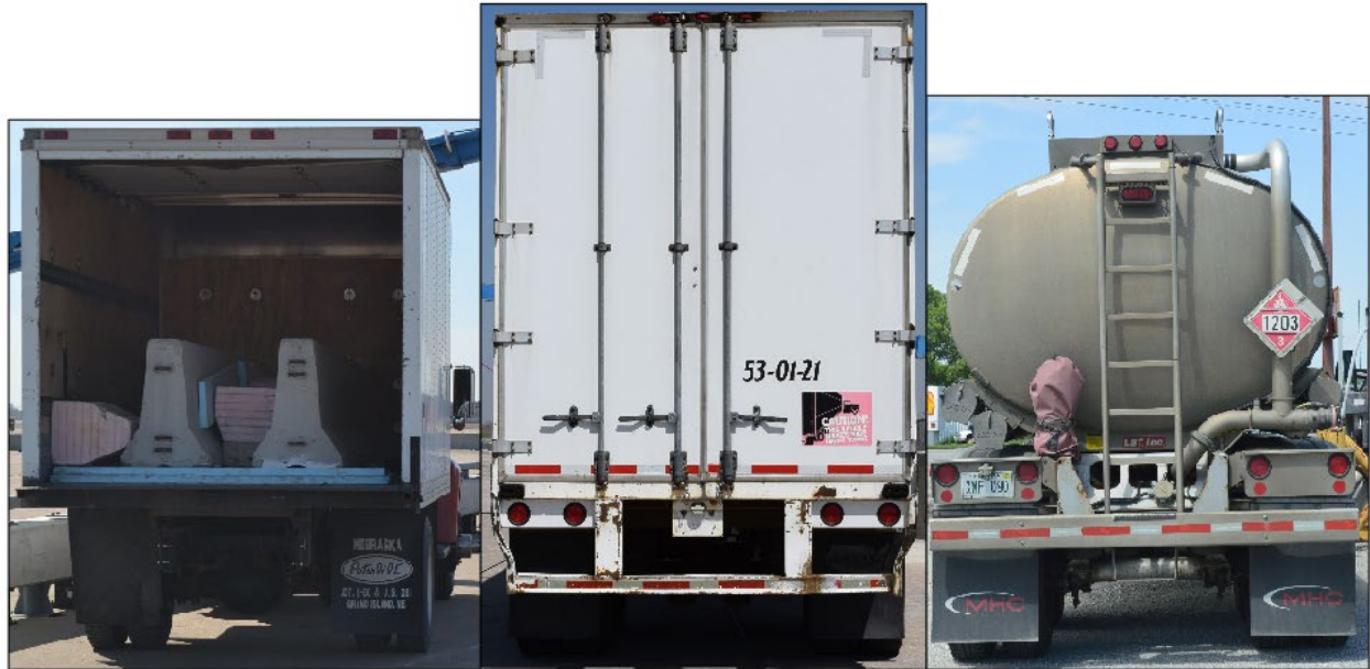
Figure 2.2 MASH Test Vehicle Back End Geometries: TL-4 (left), TL-5 (middle), and TL-6 (right)
